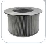
The filtration is guaranteed by an antistatic polyester cartridge filter. The cartridge is made to keep a huge filter surface in a compact space. In this way the air can pass through also when the filter is dirty. The cartridge is in M Class (BIA | En 60335-2-69) certified. It means that all particles till 1 micron are stopped by the filter so as to protect the turbine and the operator around the vacuum cleaner.
