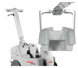
Quick, handy brush coupling and uncoupling: just press the dead man's levers three times then confirm uncoupling on the Vispa EVO display, to remove the brush.
