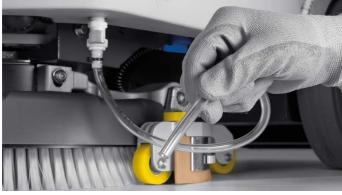
The drainage of the water from the solution tank is quick and practical, thanks to the special drainage hose that can be hooked up to the front part of the scrubbing machine.
