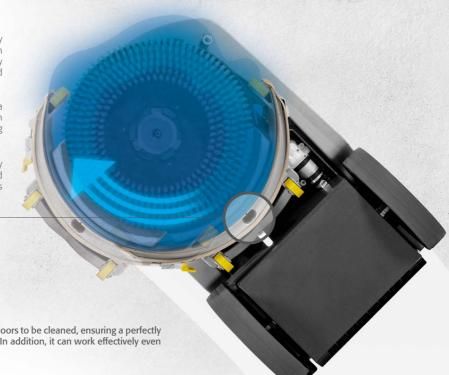
The movement of the orbital brush head enables different types of floors to be cleaned, ensuring a perfectly uniform clean, as the pad always remains in contact with the floor. In addition, it can work effectively even without the use of chemicals in many situations
