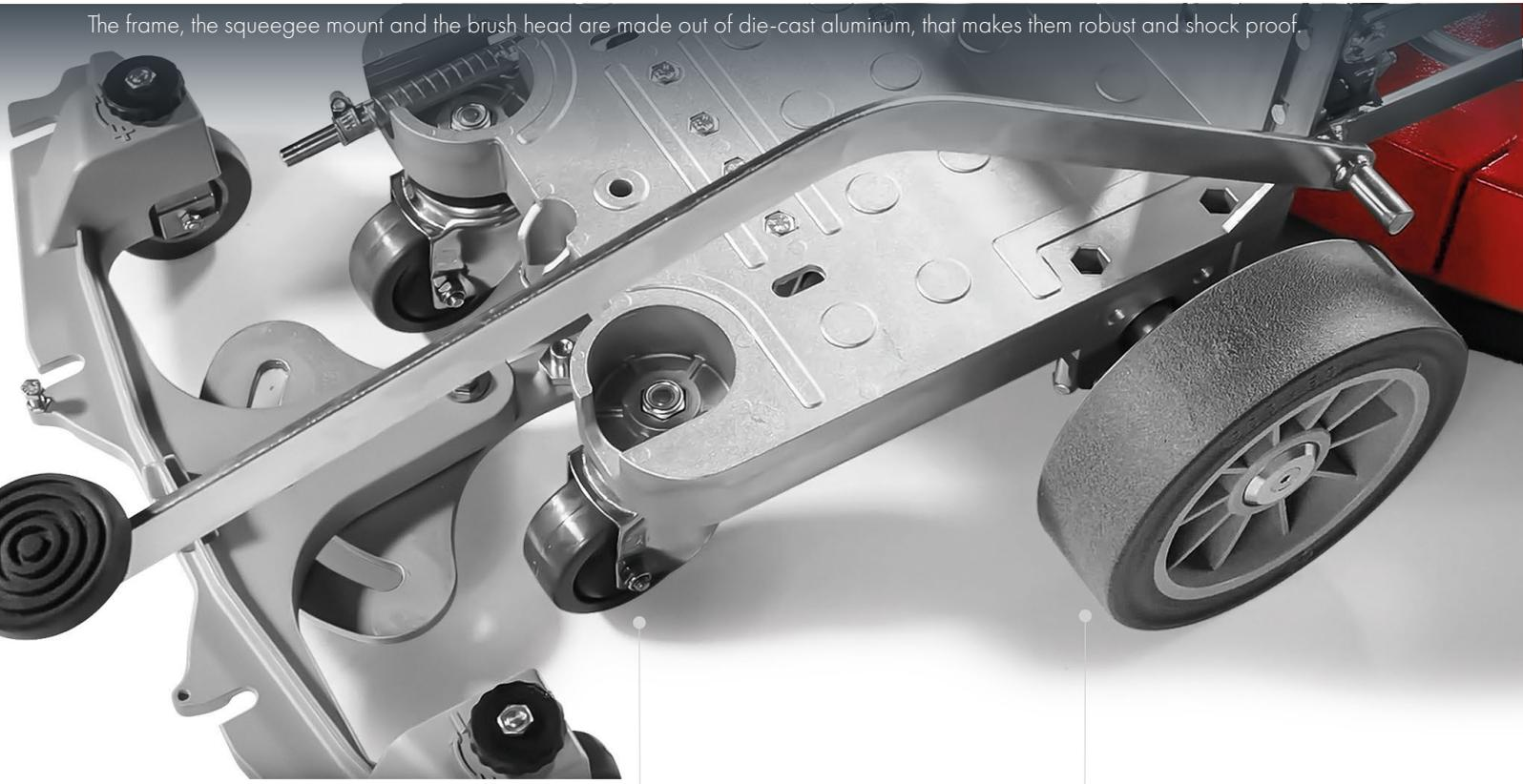
The 4 wheels increase stability and manoeuvrability. Moreover, they make brush maintenance easier and allow to store the machine with the brush head up, to keep the brush in perfect conditions.
