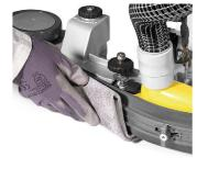
To ensure a perfect drying, the suction hose and the squeegee rubber blades must be For an effective vacuuming the suction cleaned at the end of any cleaning operation. The squeegee can be lifted to quickly clean filter must be kept clean
