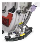
The chain to lower the squeegee is robust, made of steel, and equipped with an ergonomic handle, made out of die-cast aluminum
