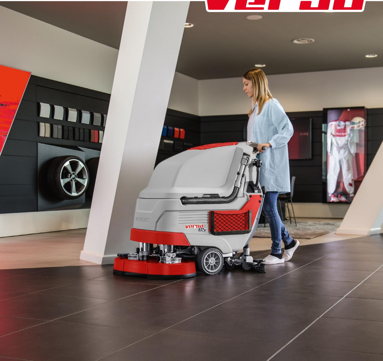
Versa is a battery powered walk-behind scrubbing machine with automatic traction, available with 2 disc brushes with 55 or 65 cm working width.
