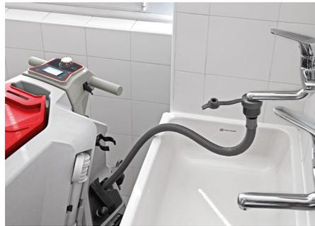
The hose for filling the solution tank can be connected directly to any water tap, thus allowing the machine to be quickly refilled at any location
