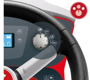
The automatic version is equipped with a **working program selector** making the use of the machine extremely intuitive. It allows to choose the selection of four pre-set working programs: Transfer, Drying, Scrubbing/Drying, Scrubbing only.
